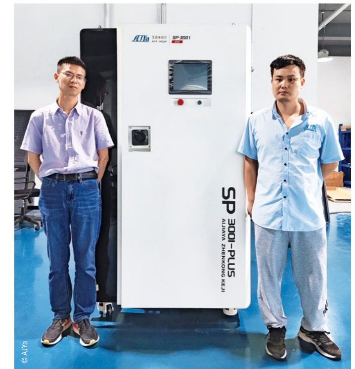
The AJYa experts Jinping Sun and Wengang Dai next to an SP series ultra-high vacuum system, where a PC-based control platform ensures optimum control of the multi-stage vacuum generation in automotive die casting machines.
